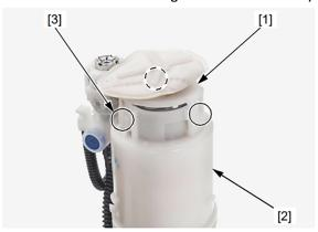
8. Disconnect the 2P connector [1] from the fuel pump/ filter assembly [2].
