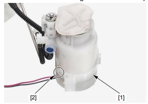
7. Remove the fuel pump/filter assembly [1] from the strainer case [2] by releasing the three tabs [3].
