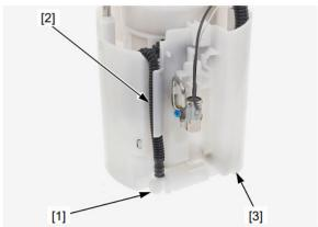
3. Push the pump flange [1] and remove the Ering [2] from the rod end. Remove the pump flange/rods from the reservoir, then remove the spring [3] from the rod. Remove the fuel pump/strainer assembly [4] from the reservoir [5] by releasing the three tabs [6].
