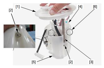
4. Insert the protruding part of the Special Service Tool (SST) in the lock tab (under the claw). Press the SST up until it clicks. Repeat this process using a second SST for the second lock tab.
