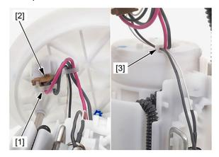
2. Remove cap A [1] and release the return hose [2] from the reservoir [3].
