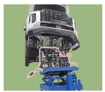
2. During the removal of the front subframe from the vehicle, loosen and unbolt the LH and RH lower control arm ball joint assemblies (A & B).
