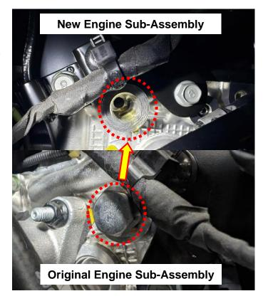
5. Install all remaining parts in reverse order of removal.
