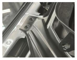
12. Remove wiper motor and linkage (Torque 12nm), pay attention to red lock tab on wiper motor plug.
