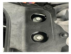
11. Remove upper support bolts (torque 56Nm)
