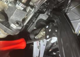
18. Release 2 retaining nuts for hydraulic unit assembly (Torque 21Nm – replace nuts).
