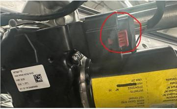
13. Unlock and disconnect/unplug DSCi Hydraulic Unit electrical connection. Red lock tab across, depress black lug, open with grey lever arm, and disconnect.
