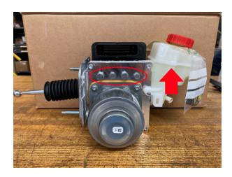
**"Wet" IB pre-filled:** Brake fluid reservoir is filled (arrow) and brake fluid line ports are plugged with bolts (circled).
