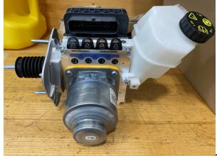
"Dry" IB unfilled: Brake fluid reservoir is empty; brake fluid line ports are sealed with labels.
