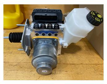
"Dry" IB unfilled: Brake fluid reservoir is empty; brake fluid line ports are sealed with labels.
