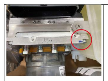
6. Verify the blue mark is located on the new component as shown in the photo.
