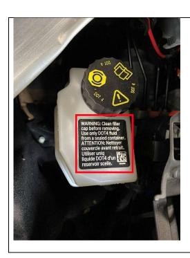
9. For G60 and G70, install the brake fluid label to the reservoir
