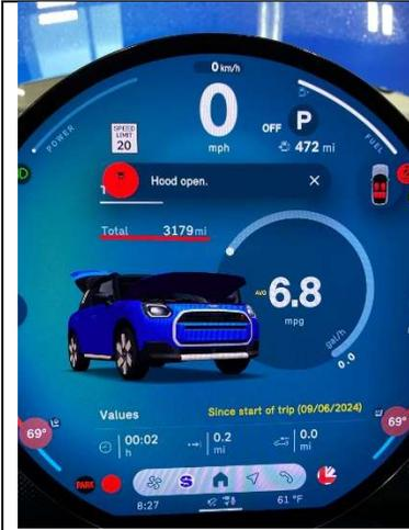
8. Note down the odometer mileage before performing the IB replacement.
