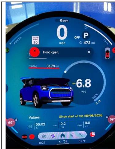
21. Document the odometer mileage in the repair order after the IB has been replaced and successfully programmed and coded to the vehicle.
