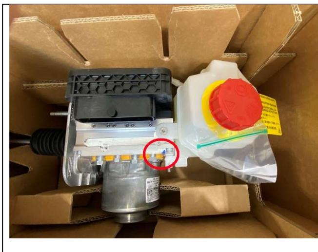
7. Verify the blue mark is located on the new component as shown in the photo.
