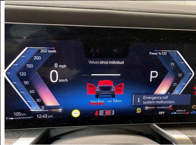
**Note:** The odometer will display 0 miles until the vehicle programming and coding is completed.
