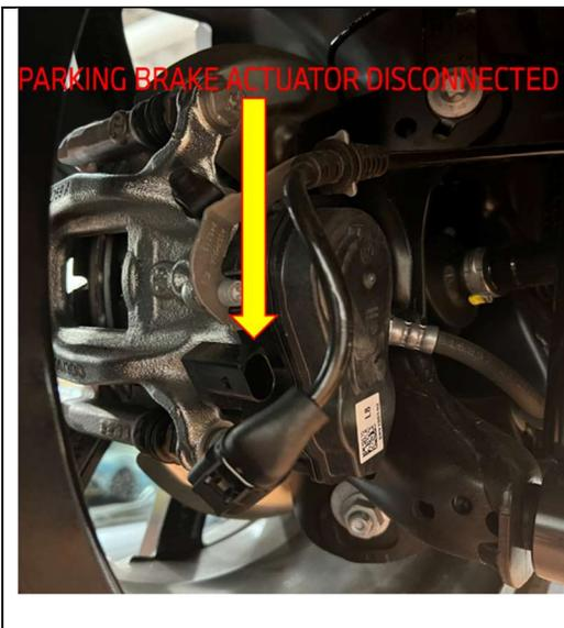
10. Disconnect the left and right parking brake actuators.
