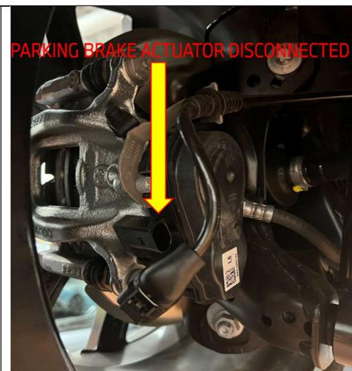
10. Disconnect the left and right parking brake actuators
