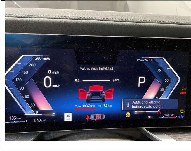
28. Document the odometer mileage in the repair order after the IB has been replaced and successfully programmed and coded to the vehicle.
