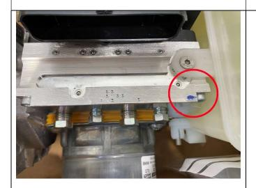
4. Verify the blue dot is located on the on the new component as shown in the photo.
