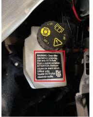
7. For G60 and G70 install brake fluid label.
