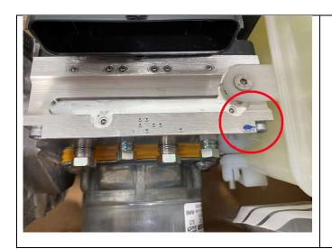
1. Inspect the IB installed in the vehicle for a blue dot as shown in the photo.
