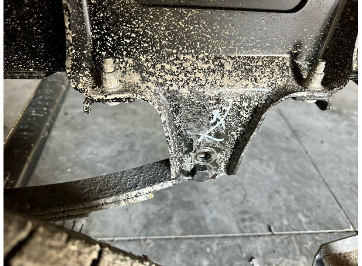
REAR, LOWER AXLE HANGER MOUNTED
