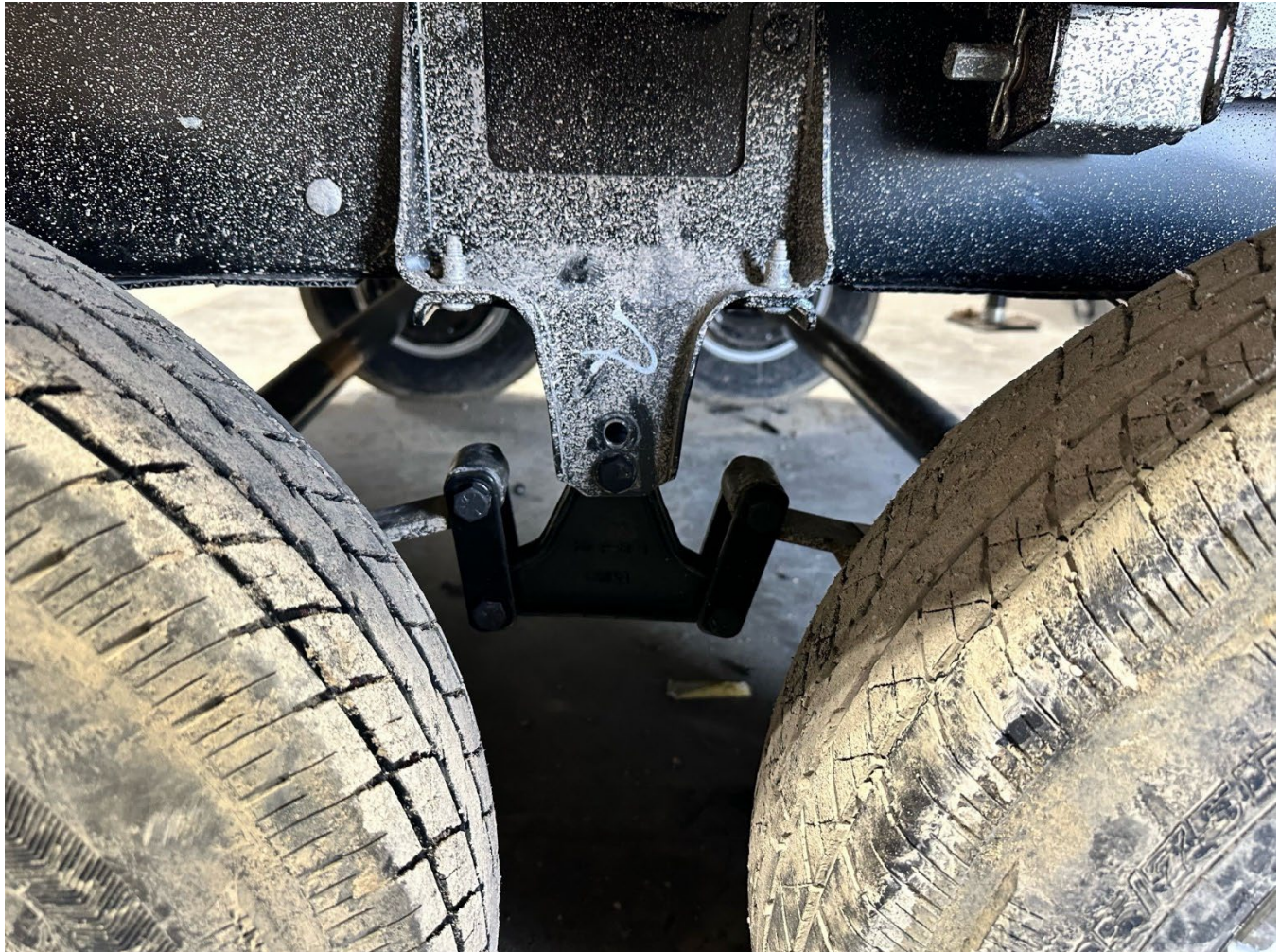
CENTER, LOWER AXLE HANGER MOUNTED WITH REPLACEMENT SHACKLES & EQUILIER
