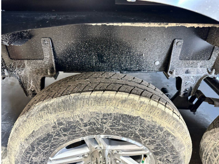
FRONT, LOWER AXLE HANGER MOUNTED
