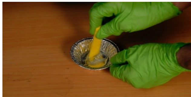
Figure 23 – Mixing the epoxy.
