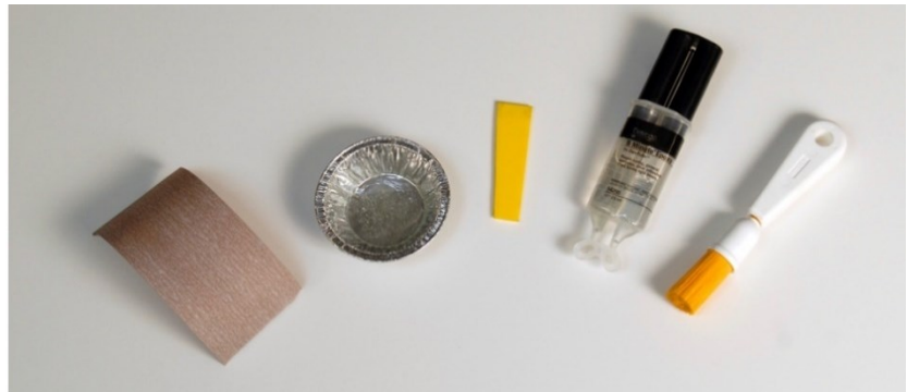
Figure 21 - Epoxy and tools needed for tank repair.
