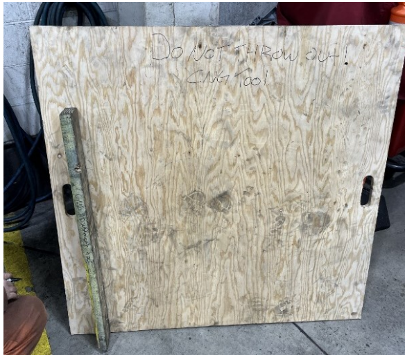
Figure 2 - Plywood frame support and CNG Driver Tool
