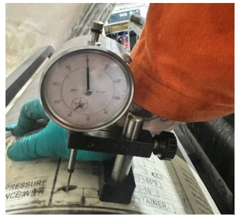
Figure 5 - Damage being measured with a dial indicator gauge.
