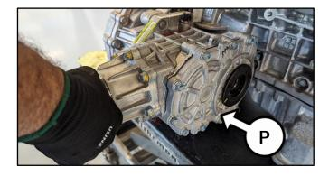
14. Separate the automatic transaxle assembly (Q) from the engine (R).
