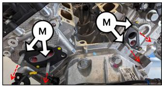
11. Remove both left <u>and</u> right side exhaust manifolds (N).
