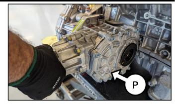
14. Separate the automatic transaxle assembly (Q) from the engine (R).
