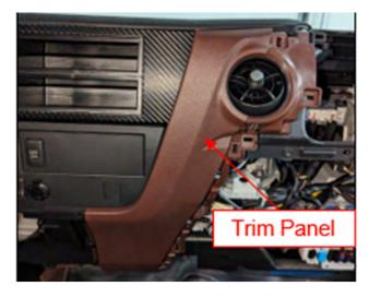
**6.** Carefully pull the trim panel piece surrounding the HVAC control panel towards the rear of the vehicle to release all retaining clips.
