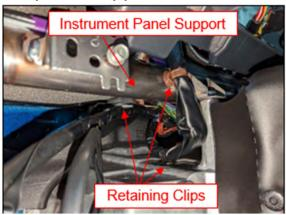
**90.** Connect the ground eyelet to the instrument panel support and tighten the bolt to the specified torque. Connect the door harness connection. Position the diagnostic connector into the mounting bracket.
