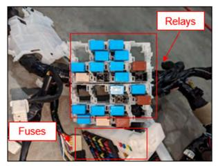
**57.** Place the new cab harness inside the vehicle and install the junction box into the bulkhead. Be sure to place the extra gasket over the lower outer bolt. Tighten the bolts to the specified torque.
