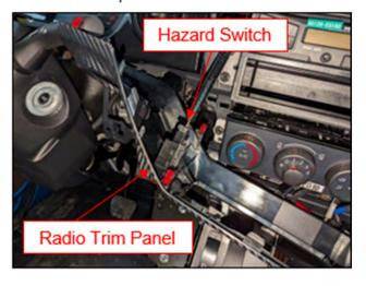
9. Lift upwards on the instrument cluster trim panel to remove.
