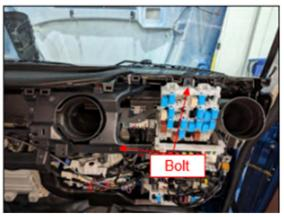
**33.** Remove the upper instrument panel cover from the vehicle. Detach the wire harness attachment clip on the underside of the radio opening while removing the upper instrument panel cover.
