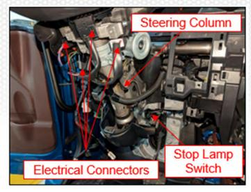
**92.** Install the steering column trim. Tighten the four screws to the specified
