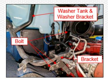
**65.** Connect the wire harness to the washer fluid pump and A/C pressure switch. Lock the harness attachment clip into the bracket and connect the
