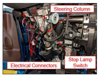
**21.** Remove the bolt securing the ground eyelet and disconnect the door harness connection. Remove the diagnostic connector from the mounting
