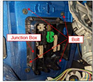
**56.** Verify the part number of the replacement cab harness when compared to the one removed from the vehicle. If correct, transfer relays and fuses one at a time from the old cab wire harness to the new cab wire harness.
