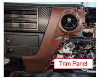
**105.** Fit the shifter console upper trim panel in place. Carefully and firmly press forwards to install. Thread the park brake control knob onto the park brake valve (air brake vehicles only).
