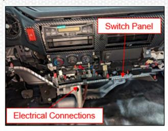
**8.** Remove the bolt securing the radio trim panel. Carefully pull the radio trim panel towards the rear of the vehicle to release. Disconnect the hazard switch electrical connector. Remove the radio trim panel.
