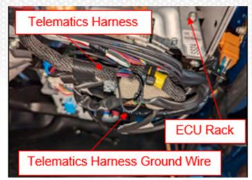
3. Slide the 300mm wire protector sleeve over the telematics harness
