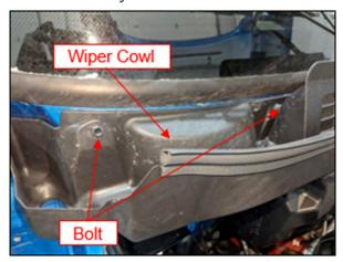
**54.** Remove the two lower wiper motor mounting bolts. Gently pull the end of the wiper cowl away from the cab, remove the two upper wiper motor mounting bolts.
