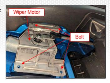
**59.** Install the two bolts in the wiper cowl and tighten to the specified torque.
