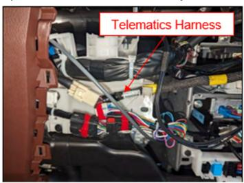
108. Route the telematics harness as shown and connect to the telematics
