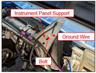
**35.** Detach the clips securing the cab harness to the instrument panel support across the HVAC case. Ensure the harness is free from the steering column and bulkhead area on the driver side of the vehicle. .
