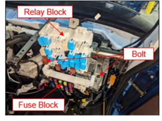
**72.** Install the upper ECU rack portion. Tighten the three bolts to the specified torque.
