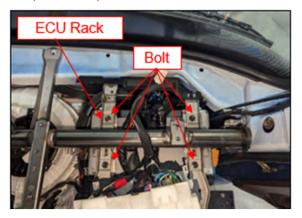
**69.** Secure the lower fuse panel to the ECU rack. Tighten the bolts to the specified torque.
