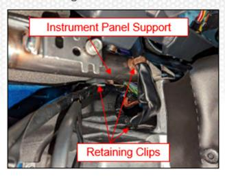
**23.** Remove the OBD2 port. Disconnect the accelerator pedal and floor harness connections.
