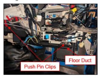
42. Remove the two bolts securing the lower fuse panel to the ECU rack.
