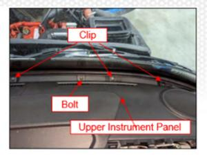
**32.** Remove the two bolts on the passenger side of the upper instrument panel cover and the two nuts on the driver side of the upper instrument panel cover.
