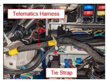
111. Install a tie strap securing the telematics wire to the cab harness at the
