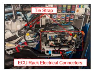
**39.** Remove the three bolts securing the upper ECU rack. Remove the upper ECU rack.
