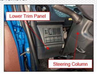
**11.** Remove the bolt securing the dimmer switch trim panel. Pull the dimmer switch trim panel towards the rear of the vehicle to release. Disconnect any electrical connectors. Remove the dimmer switch trim panel.
