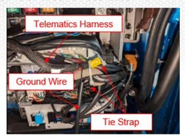
110. Install a tie strap securing the telematics wires to the cab harness at
