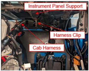
**68.** Ensuring the upper fuse and relay blocks are routed above the ECU rack, install the ECU rack. Tighten the bolts to the specified torque.
