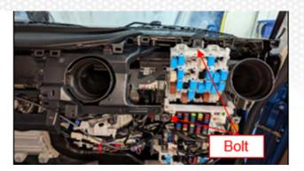
**80.** Attach the harness clip on the radio harness to the underside of the upper instrument panel.
