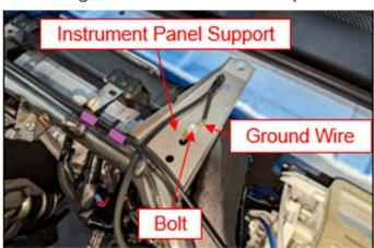
**78.** Ensure the speaker wire for the passenger side speaker is positioned correctly and place the upper instrument panel section back in the vehicle. Install the six retaining clips and two bolts. Tighten the bolts to the specified torque.
