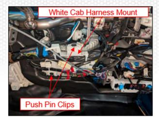
**38.** Cut the four tie straps from the harness bundle at the ECU rack. Disconnect all ECU rack electrical connectors.
