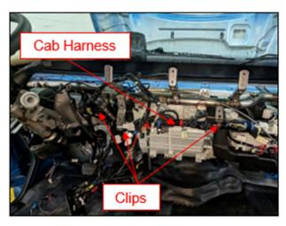
36. Disconnect the three electrical connectors on the HVAC case.
