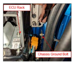
**7.** Place the new telematics harness ground eyelet UNDER the existing harness ground eyelet as shown.
