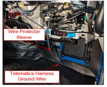
**4.** Using a 20-22AWG wire stripper, remove 7mm's of insulation from the end of the telematics harness ground wire, as shown in the photograph
