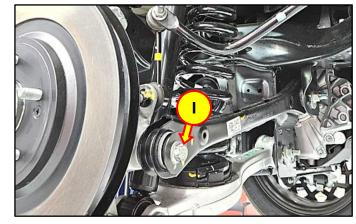
10. Remove the shock absober assembly from the vehicle.
