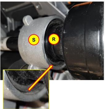
**NOT GOOD**: A gap remains between the IDA dust cover and inner shaft bracket.
