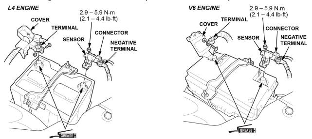
NOTE: To protect the 12-volt battery sensor connector from damage, do not hold it when installing the negative terminal.
