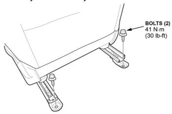
5. Slide the seat all the way back and remove the front passenger's seat mounting bolts.
