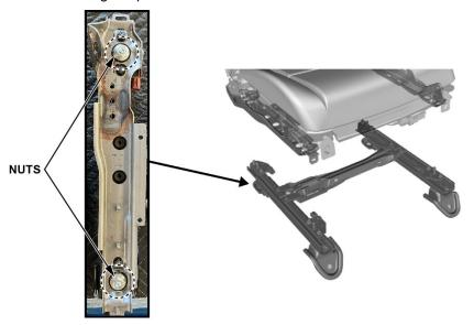
17. Mount the seat rail in the vehicle with the bolts and remove the 4 seat weight sensors, then discard the nuts and sensors.
