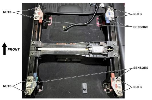
18. Install the new sensors and nuts in the orientation shown.
