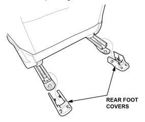
4. Remove the rear bolts of the front passenger's seat.
