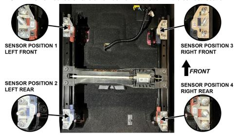
19. Place the **SWS Fixture Guide C** onto the new seat weight sensors with the tabs located on the inside of the seat track. Using the guide properly seated on the new sensors and torque the nuts to **35 N·m (26 lb-ft)** in the order shown on the SWS Fixture Guide.
