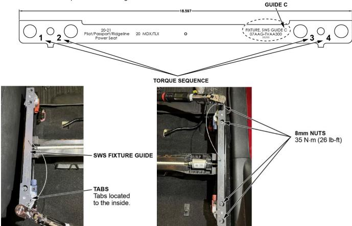
20. Remove the rail from the vehicle. Install the front passenger's seat rail back onto the seat frame, loosely install the new nuts and bolts, and reinstall all parts.
