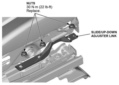
15. Remove the two bolts from the seat bracket and the two nuts, then remove the front passenger's seat rail as an assembly.
