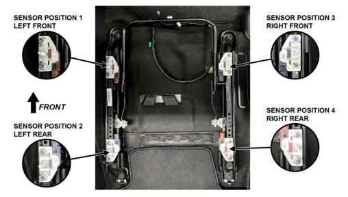
13. Place the SWS Fixture Guide E onto the new seat weight sensors with the tabs located to the inside of the seat rail. With the guide properly seated on the sensors, torque the nuts to 35 N·m (26 lb-ft) in the order shown on the SWS Fixture Guide using the socket provided.
