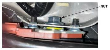
15. Use the Snap-On Torque Wrench (P/N 07AAA-TVAA400) and box-end head and torque the nuts to the specified torque **55** N·m (41 lb-ft).
