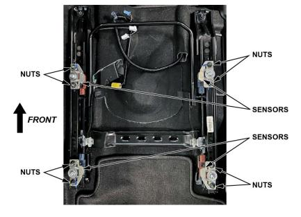
12. Loosely install the new sensors using new sensor nuts in the orientation shown.
