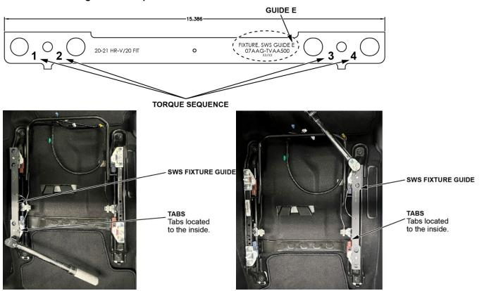
14. Remove the seat rail assembly from the vehicle and reinstall on the seat frame with new flange nuts and washers.
