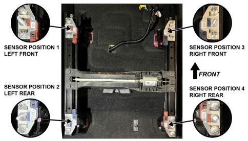
20. Place the SWS Fixture Guide B or C onto the new seat weight sensors with the tabs located on the inside of the seat track. Using the guide properly seated on the new sensors, torque the nuts to 35 N·m (26 lb-ft) in the order shown on the SWS Fixture Guide.
