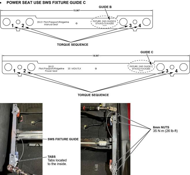
21. Remove the rail out of the vehicle.
