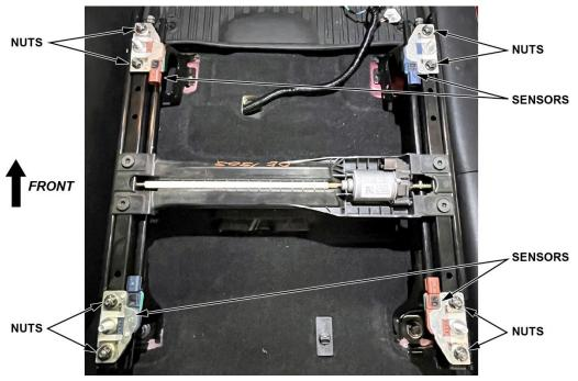
19. Install the new sensors and nuts in the orientation shown.
