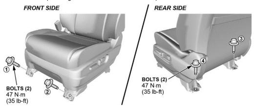
5. Move the front passenger's seat to the rearmost position and remove the front mounting bolts.
