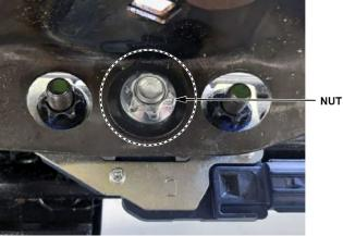
8. Mount the seat rail in the vehicle and remove the 4 seat weight sensors, then discard the nuts and sensors
