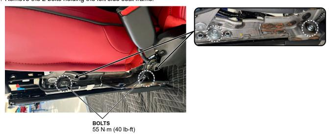
11. Remove the two bolts on the right side holding the frame.
