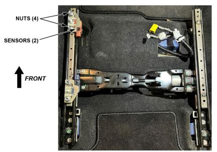
14. Loosely install the new seat weight sensors and nuts in the orientation shown.
