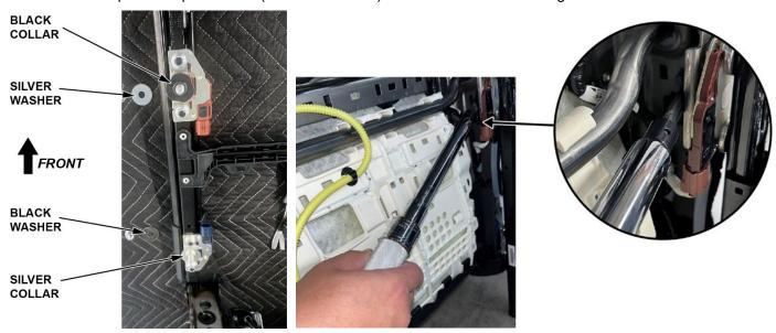
17. Install the seat and hand tighten the bolts first, then torque them in the sequence shown 43 N·m (32 lb-ft).
