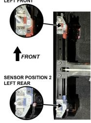
15. Place the **SWS Fixture Guide D** onto the new seat weight sensors with the tabs located to the inside of the seat track. With the guide properly seated on the new sensors, torque nuts to **35 N·m (26 lb-ft)** in the order shown on the SWS fixture guide, using the socket provided with the guide.
