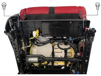
10. Remove the 2 bolts holding the left side seat frame.
