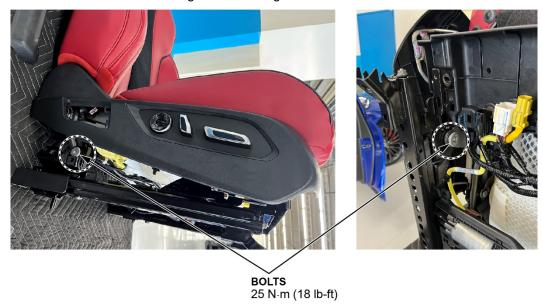
12. Remove the seat rail from the seat frame.
