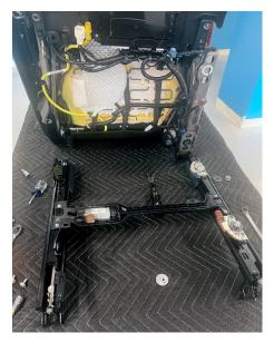
13. Mount the seat rail in the vehicle with the bolts and remove the 2 seat weight sensors, then discard the nuts and sensors.
