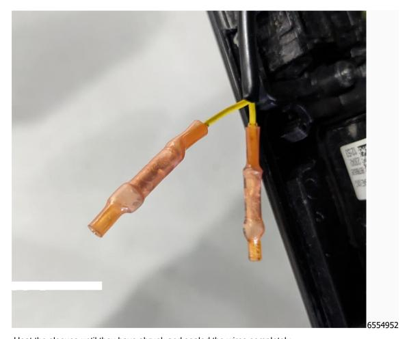
Heat the sleeves until they have shrunk and sealed the wires completely. 4.
