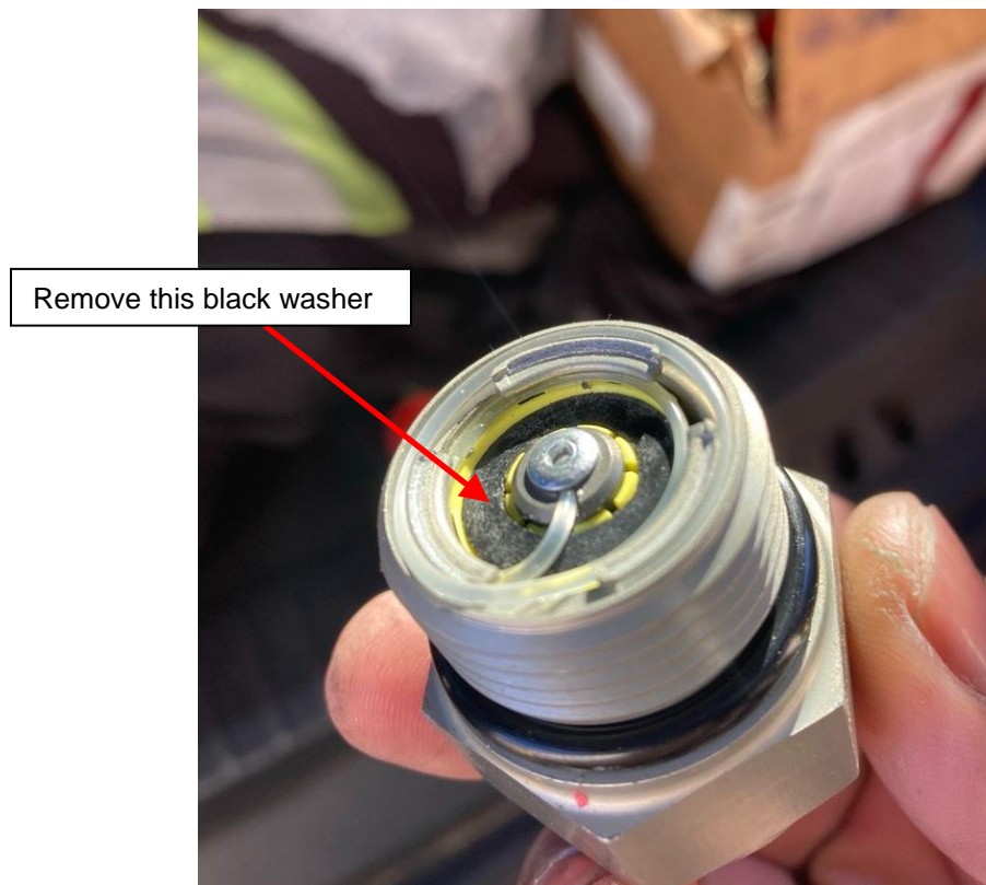
Figure 3: Remove Black Washer from Drain Cartridge
