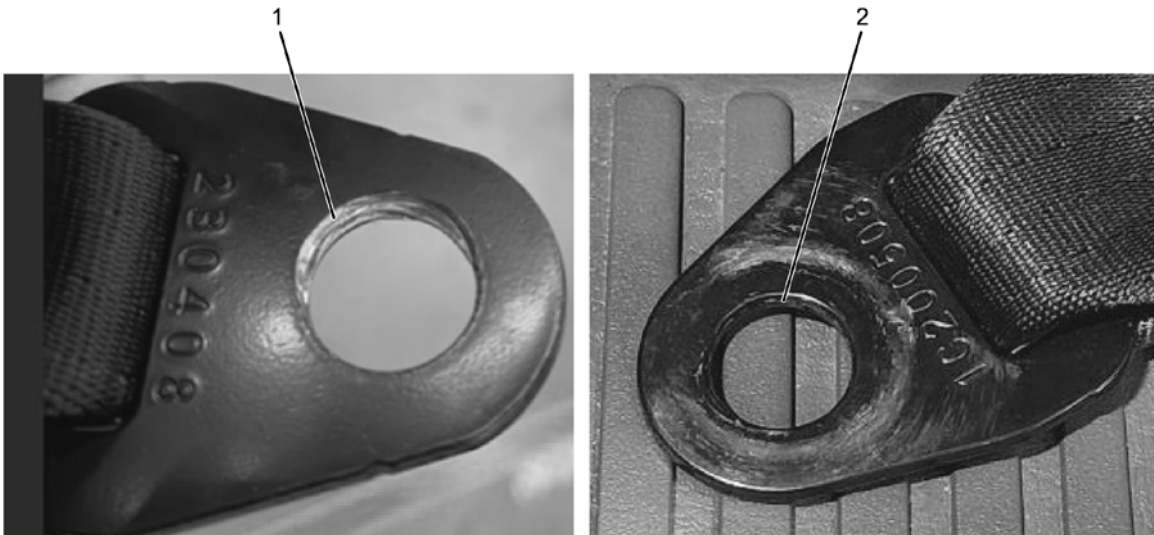
Figure 2. Tether Plate Clearance Hole at Anchor Bar
