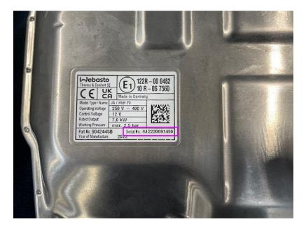
2. Replace the Coolant Heater Assembly. Refer to Water heater HVH70 GEN1.5 Remove and Replace.
