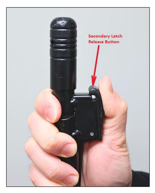
**Verification Step 2**: - After depressing the Secondary Latch Release Button three times, with the parking brake handle in the applied position, push on the parking brake handle (without depressing the Secondary Latch Release Button) with approximately 25 pounds of force to verify that the Secondary Latch is working properly.
