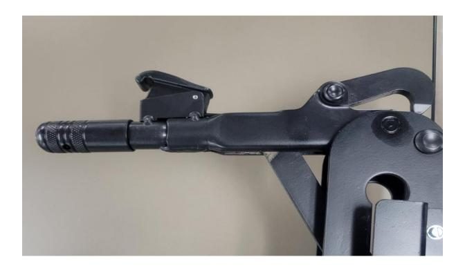
**Secondary Latch rework Step 2**: While holding the top of the lever handle in the unapplied position, push down on the back of the latch (hook) until it bottoms out. Then, release the latch (hook).
