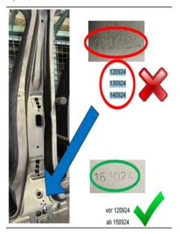
3. Check the serial number on the inner Bpillar. If the serial number is not legible, the vehicle is NOT to be sold or delivered to the customer. Continue to step 4.
