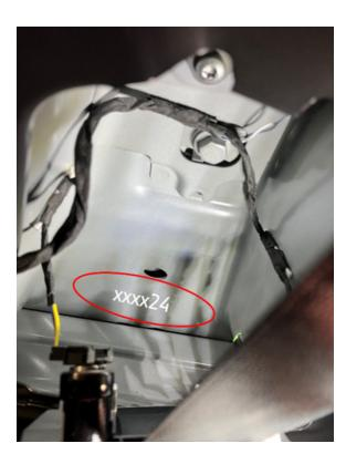
The serial number is located on the inner B-pillar in the area circled in red.
