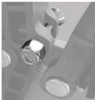
Figure 6 - An Under Torqued Fastener
