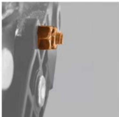
Figure 5 - An Over Torqued Fastener
