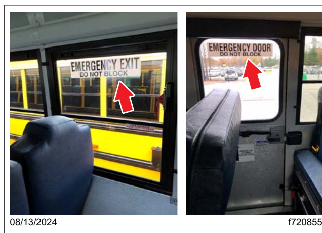
Fig. 1, Emergency Door and Window Labels
