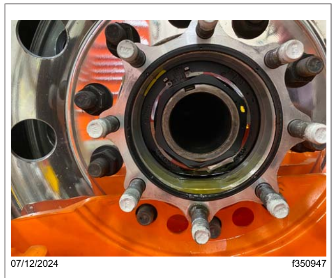
Fig. 9, Correctly Installed Locking Snap Ring
