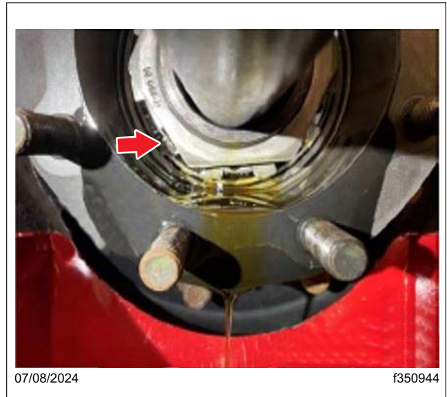
Fig. 3, Correct – Lock Tab Bent Over
