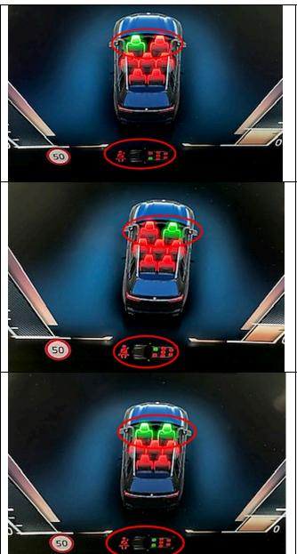
2-Here the image shows the drivers safety belt latch is recognized as latched. This should only occur when drivers' safety belt is connected / latched.
