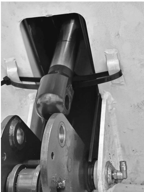
Figure 2 – Temporary support for cylinder rod end.
