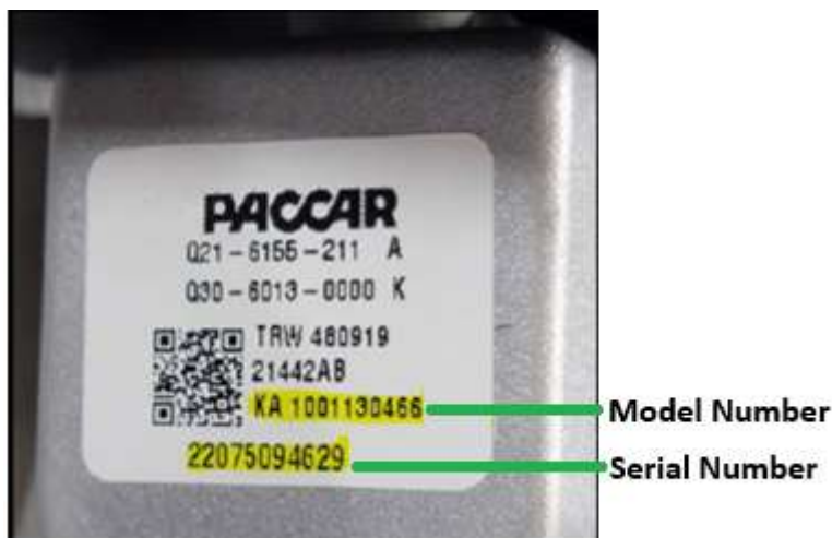
Right-hand shift stalk part/serial number label
