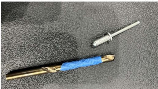
Figure 2 – 6.7mm drill bit with painters tape relative to 6.5x12.5 blind rivet - not 1:1 scale
