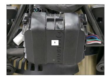
11. Remove the T-box (9) and discard the old rubber rings.
