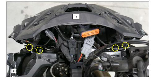
Detach the headlight housing (8) and disconnect the wiring shown with an arrow. Then remove the headlight housing.
