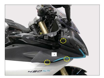
Remove screws (locations circled) for the right wing (2). Then remove that wing. Repeat for the left wing.
