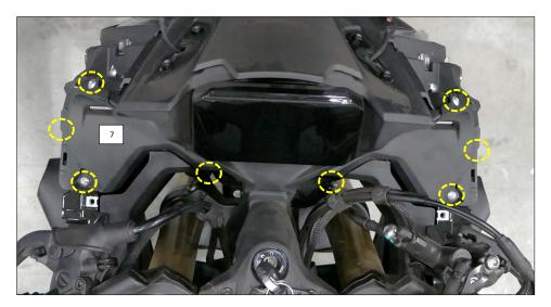
Remove screws and pushpins (locations circled) for the dashboard rear guard (7).
