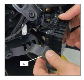
14. Slide the ring tabs over the frame bracket arms to secure the T-box to the frame. The secured T-box should sit above the T-box support bracket (11).
