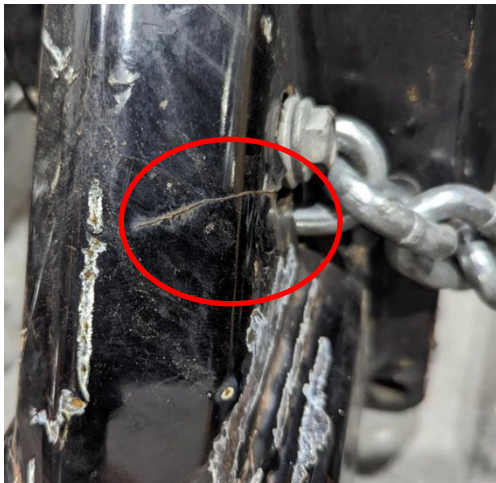
Photo 2 Example of crack near safety chain location
