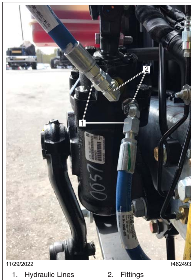
Fig. 8, Hydraulic Lines Removal
