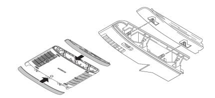
Reinstall both side panels to the side of the air diffuser.
