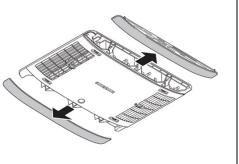
Remove both side panels on the air conditioner diffuser housing by sliding sideways.
