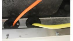
If grommet is missing, use the split to install the grommet over top of the 12/2 wire and insert into the hole in roof frame.
