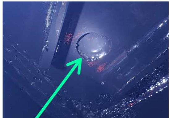
4. During inspection it's important to verify the quantity of weld applied on each hole, less than 50% or missing will need, need to follow step 16,17 & 18.
