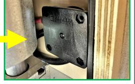
Place the post protective cover over the battery disconnect terminal posts and screw on using the 1/2" screw.
