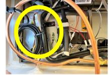
Reinstall the negative cable on to the coach batteries and resecure the wiring on the back of the fridge.
