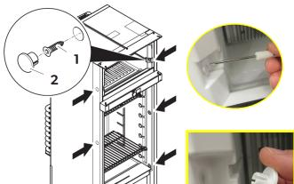
Open the refrigerator & freezer doors and remove the screw covers one side at a time.
