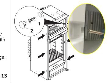
Reinstall the 6 mounting screws and caps.
