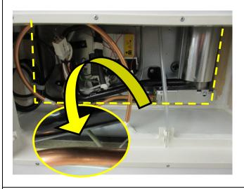
Visually check to make sure that there is no interference with the gasket and it is contacting the backside of the fridge.
