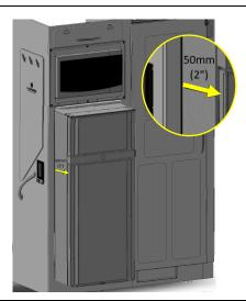
Close the refrigerator doors and pull the fridge slowly into the coach **50mm** (2") to allow access to the battery disconnect.
