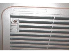
Verify fridge vent cover is secure by grasping the vent louvers and gently pulling on them to check the right side tabs engaged correctly.
