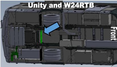
Locate the propane regulator under the floor near the rear of the coach.
