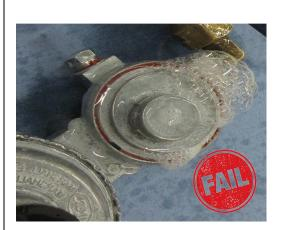
Bubbles forming indicate a detected leak and the regulator must be replaced.
