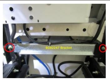
Use the 1/2" socket and wrench to remove the regulator bracket bolts.
