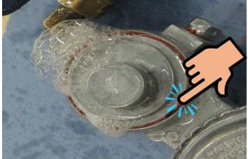
Place finger over regulator casing alignment hole (if visible) to verify excessive blowout is not preventing bubble formation.
