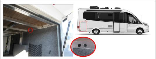
Open the rear garage compartment door and locate the double holes in the underside of the bed frame.
