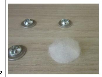
Use the metal putty knife to remove the Velcro coins covering the machine screw heads on the side being repaired.
