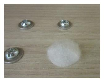
Use the Velcro coins 124-8253 to cover the machine screw heads.
