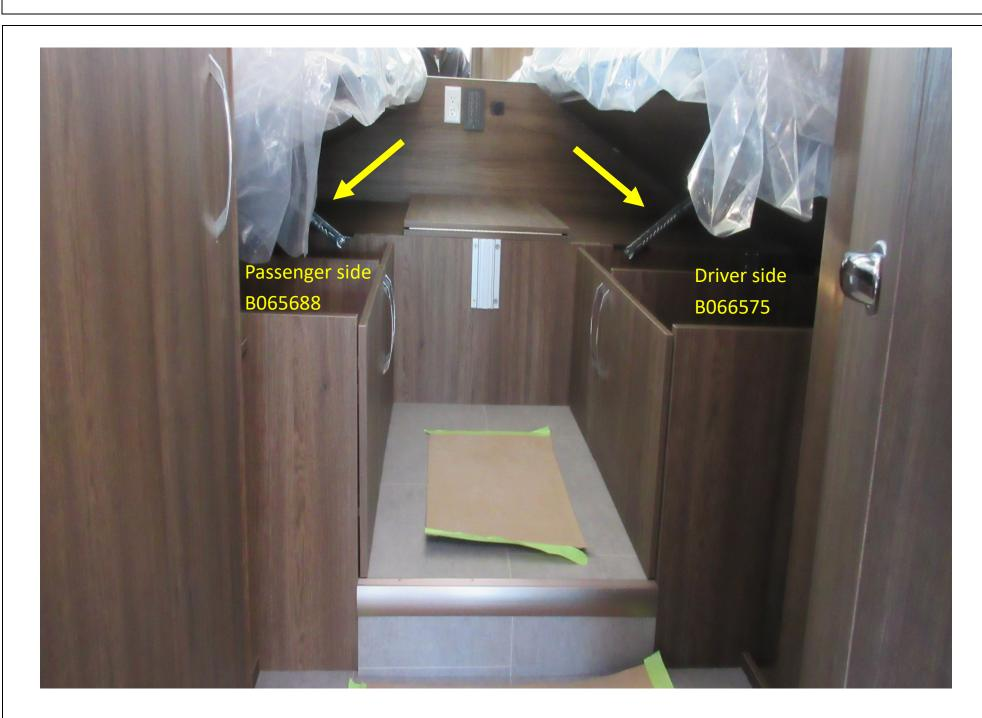
Open both bed lids to locate the ratcheting bed stay and inspect the bed stay focusing on the ratcheting mechanism.
