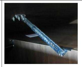
Replace the bed stay with the correct version. with the notch to the bottom and the teeth pointing up.
