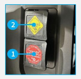
c. Pump the brake pedal until the system air pressure drops to under **60 psi (413.7 kPa)**.
