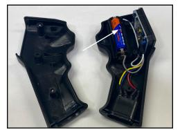
AWARNING If corrosion is observed on the circuit board or battery pack, <u>DO NOT USE</u> the remote. Contact Warn Industries' customer service for a replacement.
