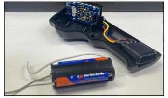
Replace remote control cover and the three screws.
