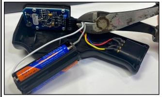
Remove and discard battery pack completely.
