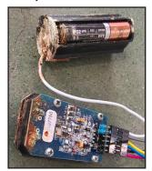
Cut the grey and white wires to release the battery pack from the remote.
