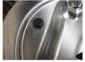
3. Using a #2 Phillips screwdriver, loosen the screws under each bumper. This will retract the clamping mechanism that attaches the cooktop to the countertop.
