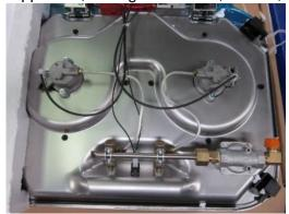
7. Clean bottom of main top near regulator with a 50/50 mixture of rubbing alcohol and water.
