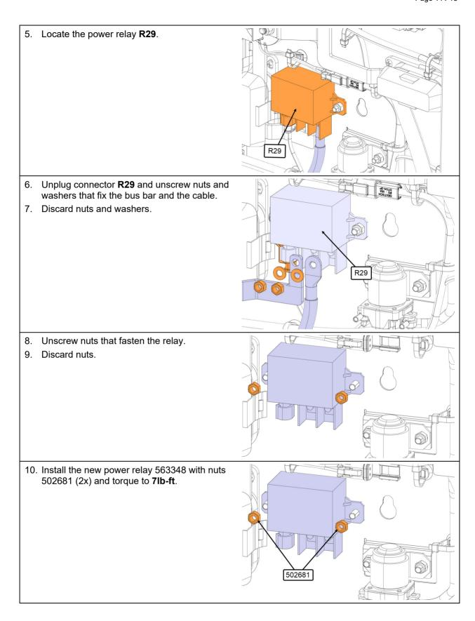
11. Plug connector R29 and fasten the bus bar and the cable to the power relay with nuts 502681 (2x) and flat washers 502573 (2x). 12. Before to apply the final torque, verify the cable does not touch the bus bar. 13. Tighten nuts to a torque of **60lb-in**. 14. Apply torque seal on nuts. 60lb-in 15. Switch on main circuit breakers CB2 & CB6. CB6 CB2 17. Close rear junction box door.
