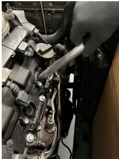
PISTON STOPPER P/N 07AAB-5G0A200
