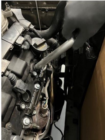
PISTON STOPPER P/N 07AAB-5G0200
