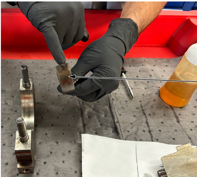
BEARING Lubricate the bearing prior to insertion.
