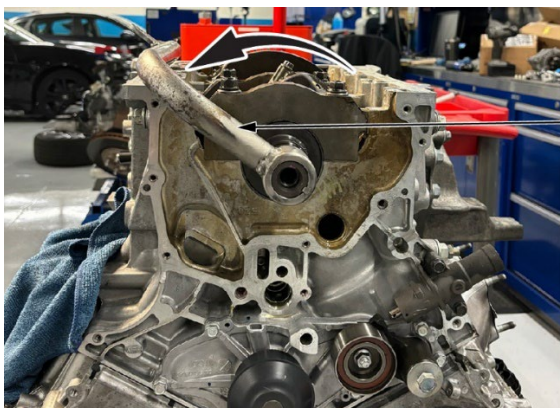
HANDLE Push the handle this direction.
