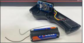
With battery pack removed, replace the remote control cover and the three screws.
