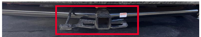
TOW HITCH HARNESS INSTALLED
